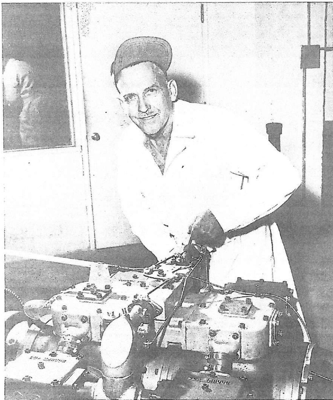
THE BOURKE 400 CAN BE TOP OVERHAULED IN TWO HOURS USING ONLY A FIVE - SIXTEENTH ALLEN WRENCH
